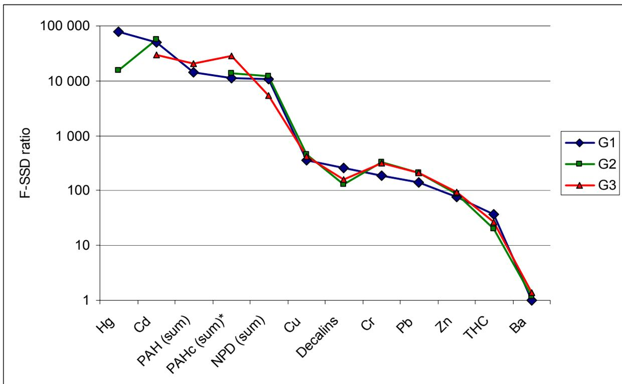
**Fig. 5.4:** Comparison of adjusted F-PNECs derived from F-SSD using bootstrap method: G1= Dataset 2 a (“mud”), G2 = Dataset 2b (“mud - fine sand”), and G3 = Dataset 2c (“fine sand – sand”). The data are normalized for F-PNEC for Ba in Dataset 2a (F-PNEC<sub>x</sub> = 2645 mg/kg). Note the scale: 1 – 100.000.
