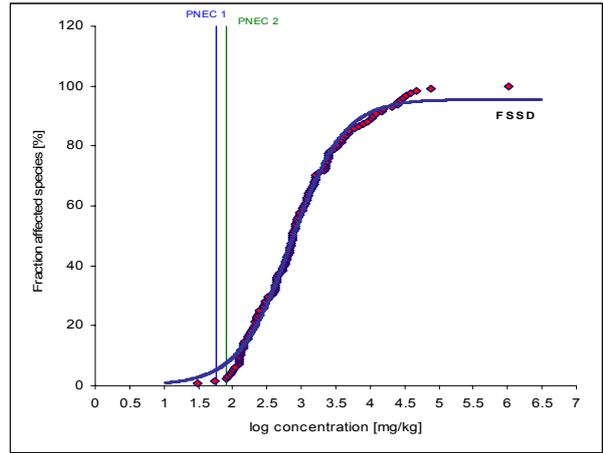
**Figure 8.3:** F-SSDs for dataset 3 (grain size interval 1 → “mud”) using bootstrap method. The solid line shows the median estimate (50%) percentile with lower (5%) and upper (95%) percentiles (dashed lines), which constitutes a 90% two-tailed percentile confidence interval. The apparent 5 % protection level and the adjusted 5 % community level are shown as lines in each figure.
