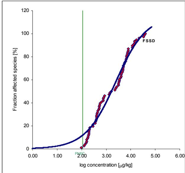
**Figure 8.7:** F-SSDs for dataset 5 (grain size interval 3 → “fine sand –sand”) using bootstrap method. The solid line shows the median estimate (50%) percentile with lower (5%) and upper (95%) percentiles (dashed lines), which constitutes a 90% two-tailed percentile confidence interval. The apparent 5 % protection level and the adjusted 5 % community level are shown as lines in each figure.
