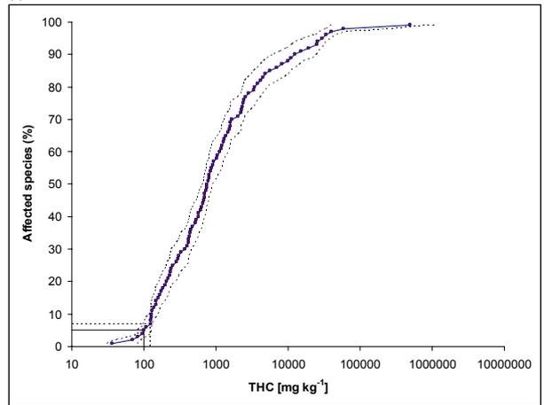
**Figure 8.2:** F-SSDs for dataset 1 (common species) using logistic function. The solid line shows the logistic curve and the blue and green lines indicate the apparent 5 % protection level and the adjusted 5 % community level.
