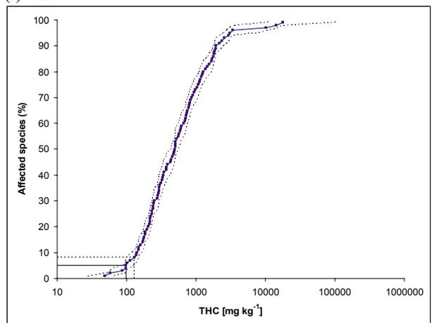
**Figure 8.6:** F-SSDs for dataset 3 (grain size interval 1 → “mud”) using logistic method. The solid line shows the logistic curve and the blue and green lines indicate the apparent 5 % protection level and the adjusted 5 % community level.
