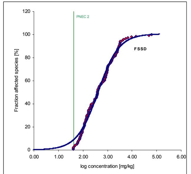
**Figure 8.5:** F-SSDs for dataset 4 (grain size interval 2 → “mud – fine sand”) using bootstrap method. The solid line shows the median estimate (50%) percentile with lower (5%) and upper (95%) percentiles (dashed lines), which constitutes a 90% two-tailed percentile confidence interval. The apparent 5 % protection level and the adjusted 5 % community level are shown as lines in each figure.
